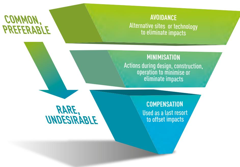
Figure 199 - The mitigation hierarchy at project level
