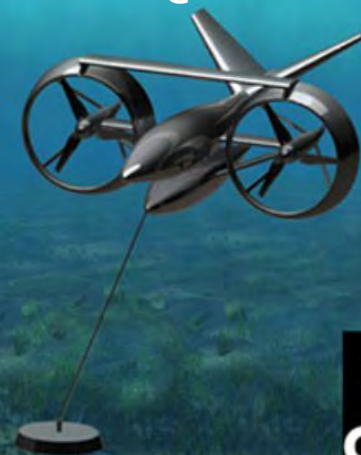
Hydrokinetic horizontal marine turbine GEM @ SEAPOWER
