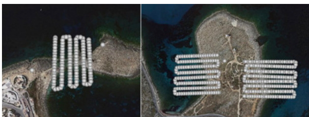
Drone transects implemented to monitor beach marine litter in Malta as part of the AMAre project.
