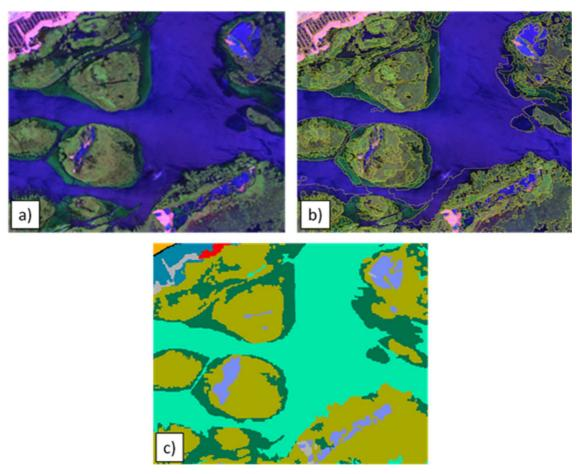
Figure 48 : Supervised and object-oriented classification of Landsat images. a) pre-processed images (input data); b) image segmentation based on spectral signatures of each pixel (including spatial, spectral and temporal variables); c) final land use map obtained after automatic classification and manual error correction (source: Tour du Valat, 2016)
