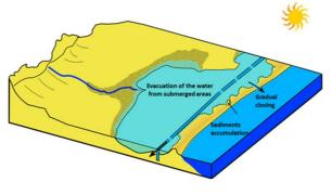
Figure 20: Sequential diagram of a storm over the Etang de Vic lagoon
