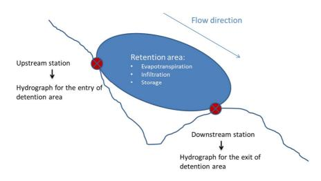
Figure 34: Diagram showing the hydrograph method: comparison of retention area input and output hydrographs
