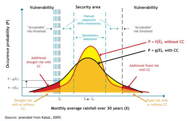
Figure 3: Effect of climate change on the probability function of a hydrological variable (here, average monthly rainfall, calculated over 30 years) and its consequences in terms of water security
